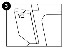
After the lid tab is inserted, gently squeeze both black side-tabs together allowing for the tabs to be inserted into the box. When the lid is secured the black side-tabs will expand into place.
