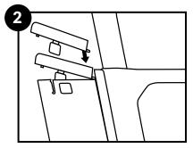
Insert the lid tab into the molded slider by angling the lid down into the lid tab hollow located just above the box.
