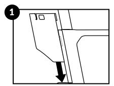
Insert the box, without the lid, into the molded slider track on the back of your seat tube. Slide the box to the very bottom of the slider.
